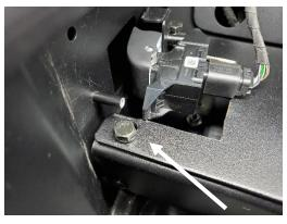
Attach mounting platform to cross braces using (4) 5/16 x 3/4" bolts, split lock washers and flat washers. Attach emergency brake release to side of console.
