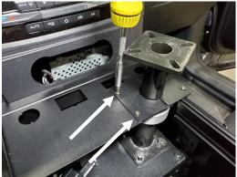
Using (4) #8 x 3/8" Torx screws, attach half-moons to top of HDM plate.
