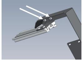
Attach extrusion and bracket assembly to HDM top plate studs using 8-32 Keps nuts.
