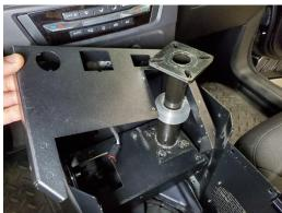
Place assembled HDM top plate onto console and line up to side screw holes in console housing.
