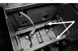
Install cross front and rear cross brace to side mounting brackets using (4) 1/4" x 1/2" carriage bolts and serrated nuts.
