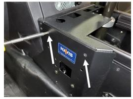
Attach top plate using #8-18 x 1/4" Phillips flat head screws.
