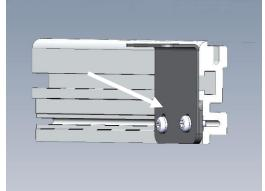
Attach console extrusion bracket and spacer to extrusion using two (2) #8 x 3/8" Torx screws.
