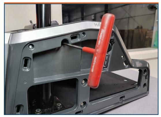
Attach Shaft collar to brace with 1/4" x 3/4" bolt, split lock washer, and flat washer. Tighten all pole mount hardware.
