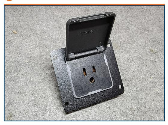
Using EXTREME CAUTION, install OEM 12v socket into relocation panel. Ensure metal tabs are in proper location.
