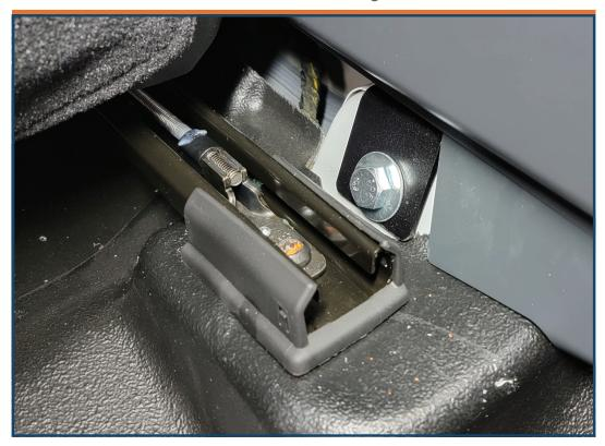
Loosely attach middle console brace to equipment mounting tray using 5/16" x 3/4" bolts, split lock washers, and flat washers.
