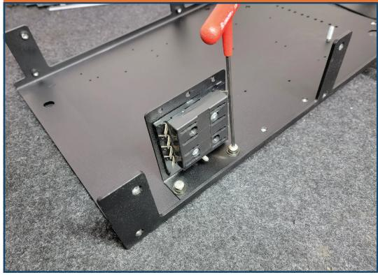
Place lower equipment mounting tray onto transmission tunnel.
