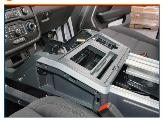
Loosely install M12 bolts and flat washers on rear, passenger seat mounting holes.
