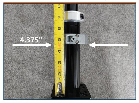
Position Clamp collar bolt and Shaft collar threaded hole to be square to flat side of pole base.
