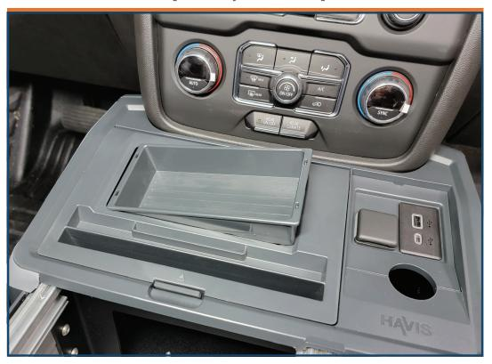
Slide pocket into opening in forward section of console. It should snap into position.
