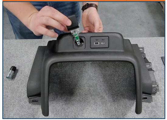
Remove OEM AUX panel from lower IP.
