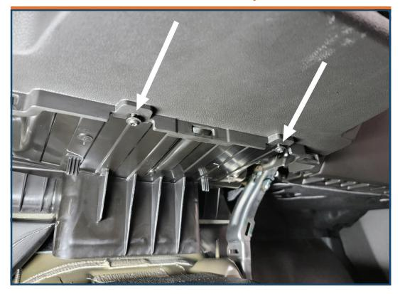
Pull lower dash panel towards rear of vehicle. Unplug harnesses and remove panel.
