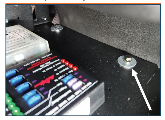
Loosely install M12 bolt and flat washer into forward seat mounting hole.
