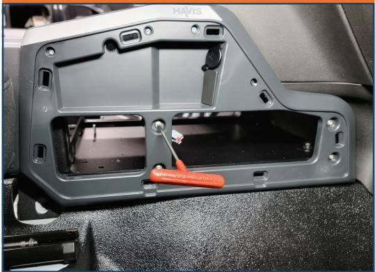
41 Use supplied mounting bracket for OEM 110V AC Receptacle.
