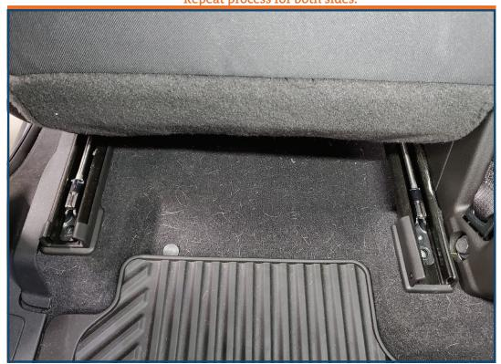
After the OEM center seat is removed, the driver and passenger seats can be bolted back in.
