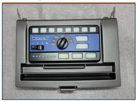
Mount control head using supplied hardware and spacers.
