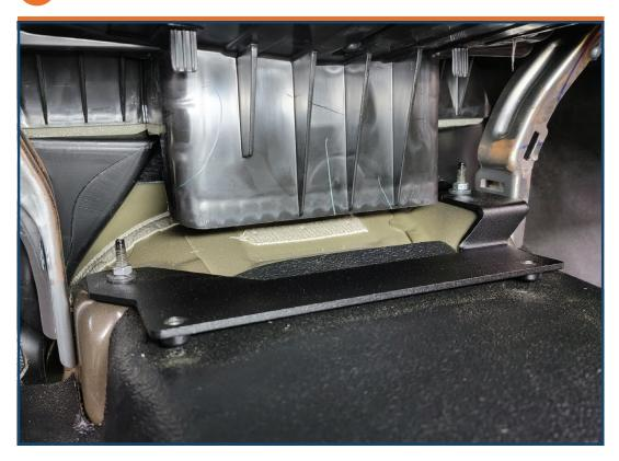
Attach using M6 nuts and 1/4" split lock and flat washers.
