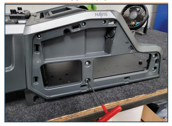
Lift off console housing from equipment mounting tray.
