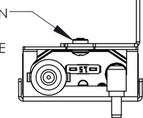
CABLES CAN FACE EITHER DIRECTION AND MOUNTED TO EITHER SIDE OF THE DOCKING STATION PENDING THE END USER'S PREFERENCE
