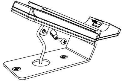
3. INSTALL VERIFONE E285 INTO ENS PROVIDED BATTERY COVER AND SECURE USING PROVIDED M3 X 4MM SCREW
