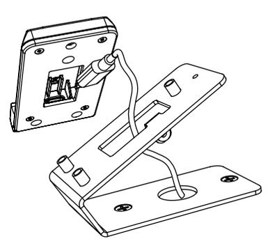
2. ASSEMBLE PLASTIC SLED TO STAND AND SECURE USING PROVIDED 3X 6-32 PHILLIPS FLAT HEAD SCREWS
