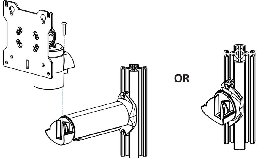
**Step 2:** Attach your VESA Monitor to the Double Pivot Mount using the 4x M4 x 10mm Phillip Screws as shown
